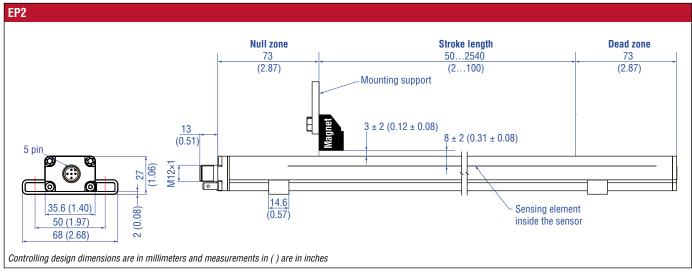
Fig. 3: E-Series EP2 with block magnet
